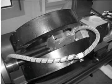
Figure 12 : measurement setup using generating coils
