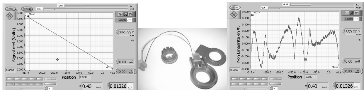
Figure 6: Prototype for steering application with output voltage and linearity for 359° stroke
