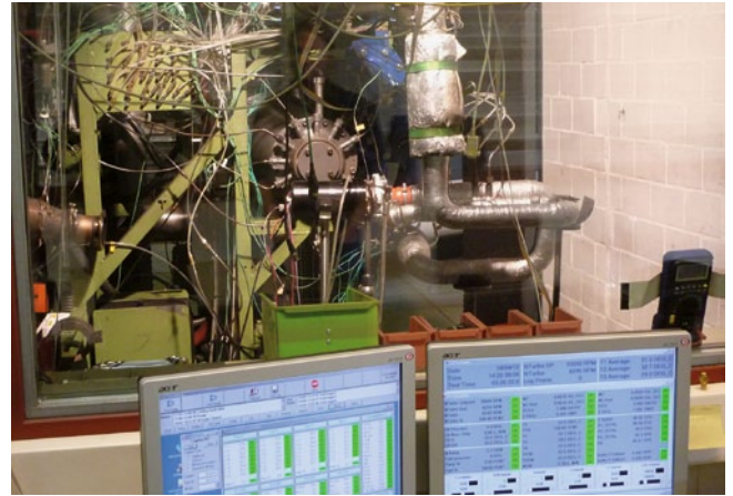
4 The compressor as set up on the test bench
