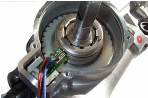
Figure 22: Picture of a prototype torque sensor integration
