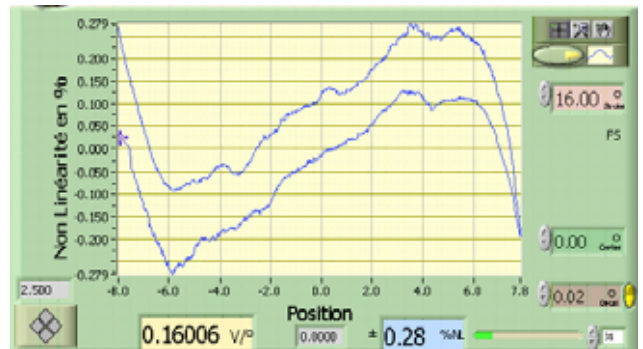
Figure 12: Non-linearity and hysteresis measurement over the stroke
