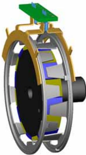
Figure 10: Optimized MMT torque sensor magnetic structure
