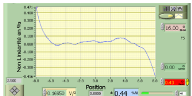
Figure 13: Non-linearity optimized on the middle of the stroke
