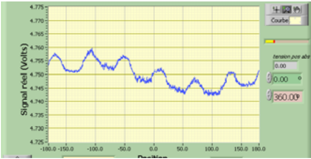
Figure 15: Stability on one turn at maximum torque position
